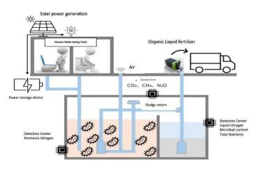
Etarn's Smart Toilets technology uses patented bacteria and micro-nano bubble-generating nozzles (activators) to turn excrement into liquid fertilizer, reducing greenhouse gases. With the integration of cloud computing and carbon credit measurement, this toilet not only improves the environment, but also creates a valuable asset.
